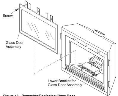
Figure 43 - Removing/Replacing Glass Door
